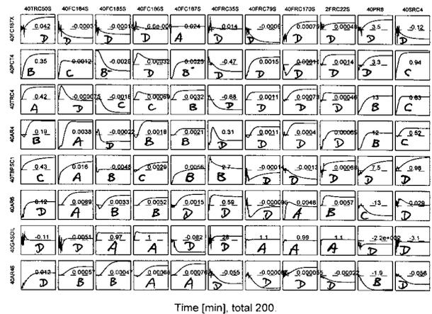
Figure 4.3 Step responses of the models of 8 CVs from Test 1
