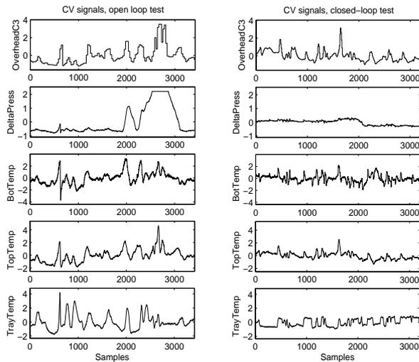
Figure 4.6 CV plots of the open loop test and closed-loop test. The data are normalised. For each output, the same scaling factor is used for both open loop test and closed-loop test.
