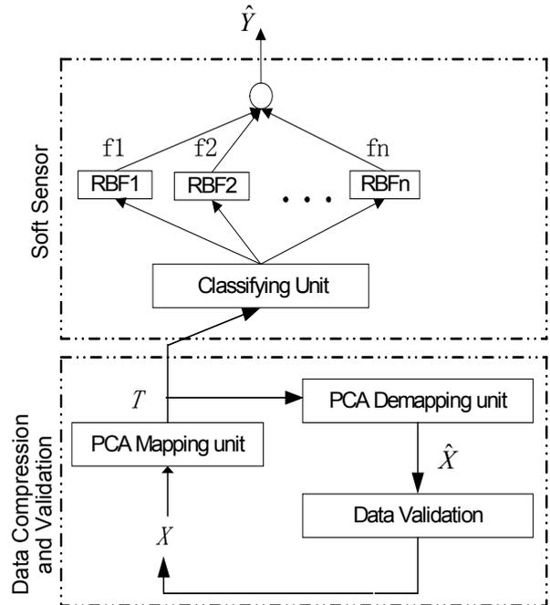
Fig. 2. Soft Sensor Structure Based on the PCA-DRBFN
