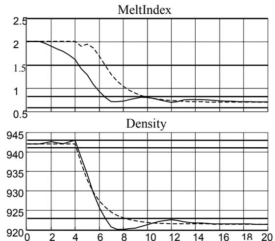
Figure 6 Trajectories for quality variables Density and Melt Index (together with specification boundaries): initial trajectory (--- , final trajectory (solid).
