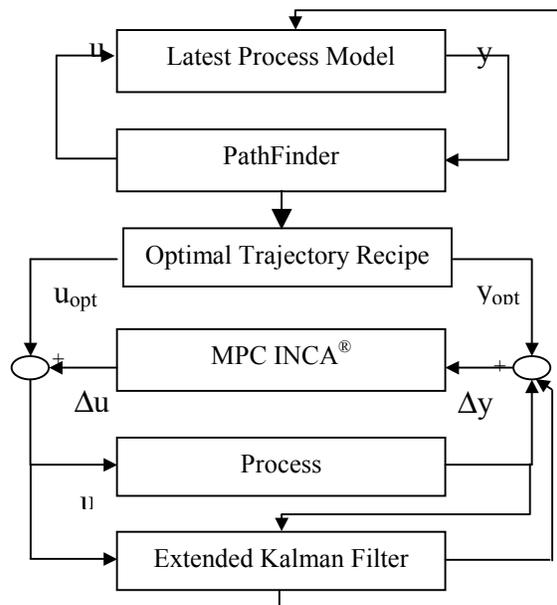
Figure 3 Integration of MPC control technology and optimization technology
