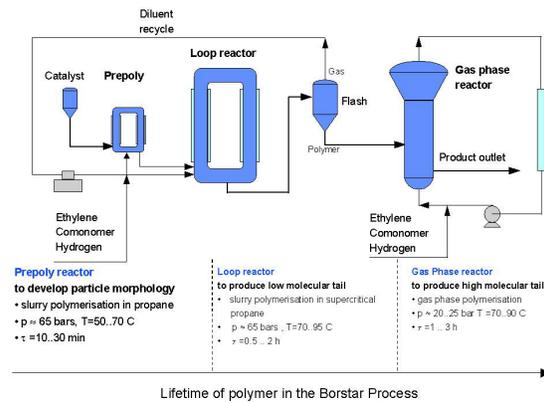
Figure 5. The Borstar process for producing bimodal MWD polymer as well as variation in co-polymer distribution.
