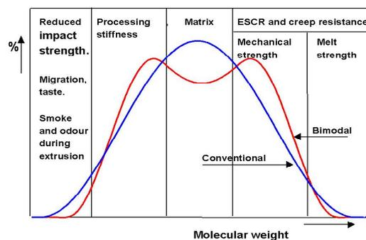
Figure 4 Molecular weight distribution can be more easily adapted with bimodal than unimodal materials to meet the property needs of the end application.
