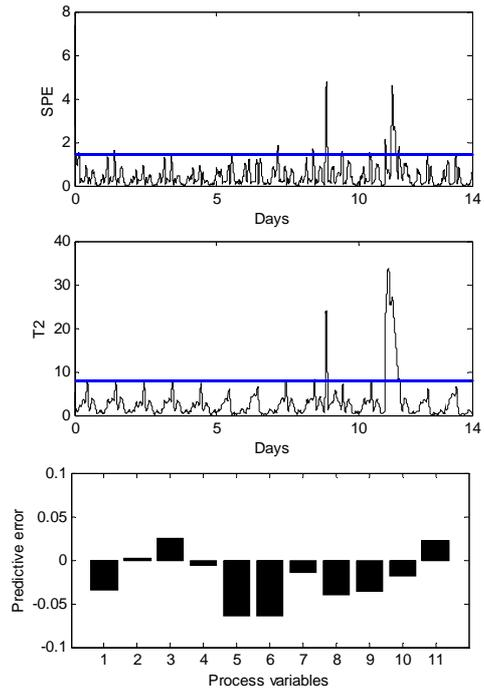
Fig. 1 monitoring storm events by PCA combined with respirometry estimations: indexes
