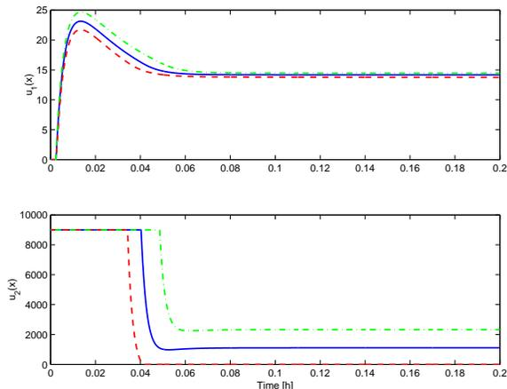
Fig. 3. Simulation of Van der Vusse reactor showing the inputs. Nominal parameter set is shown with whole lines, set 1 is dashed, set 2 is dash-dotted.
