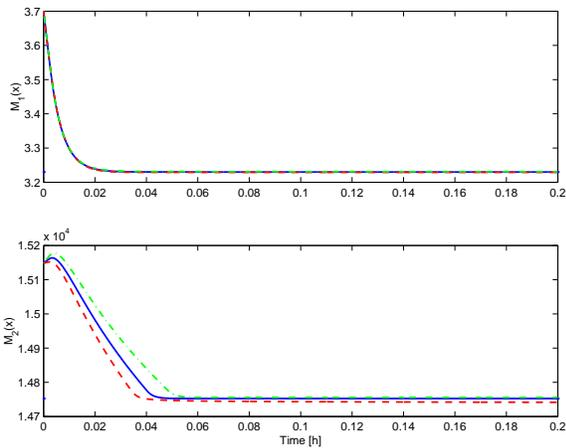
Fig. 2. Simulation of Van der Vusse reactor showing the masses of the phases. Nominal parameter set is shown with whole lines, set 1 is dashed, set 2 is dash-dotted.
