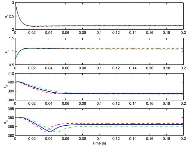
Fig. 1. Simulation of Van der Vusse reactor showing the states, from initial condition  $c_A = 3.0$ ,  $c_B = .70$ ,  $T = 400$  and  $T_K = 390$ . Nominal parameter set is shown with whole lines, set 1 is dashed, set 2 is dash-dotted.
