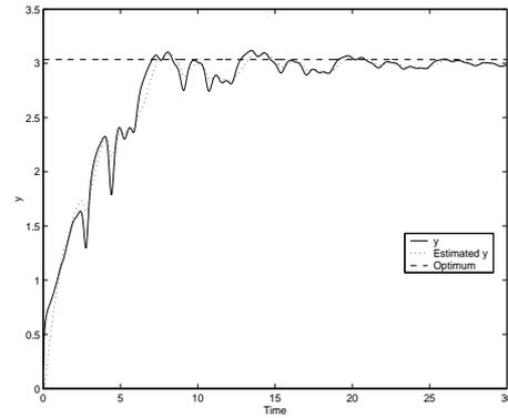
Fig. 1. Production rate  $y$  ("—") and its maximum  $y^*$  ("- -")
