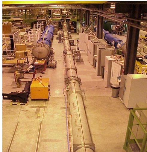
Fig. 1 Inner Triplet Prototype (length: 30 meters)
