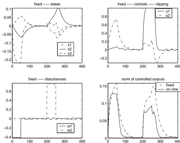
Fig. 3. Responses for fixed controller and comparison of disturbance attenuation with moving horizon controller.
