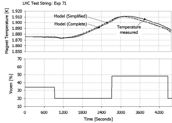
Fig. 4 Simplified vs. Complete first principles model
