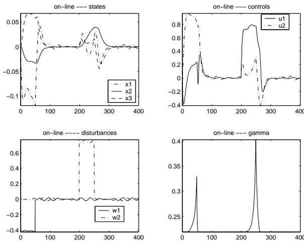
Fig. 2. Responses for moving horizon controller.
