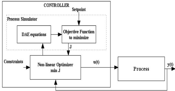
Fig. 5 Nonlinear controller – Continuous implementation framework
