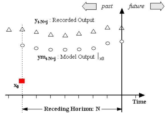
Fig. 6 Receding Horizon State Estimation
