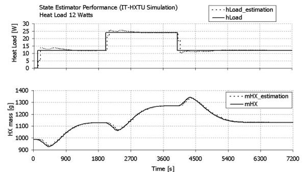
Fig. 8 Performance of the Nonlinear State Estimator
