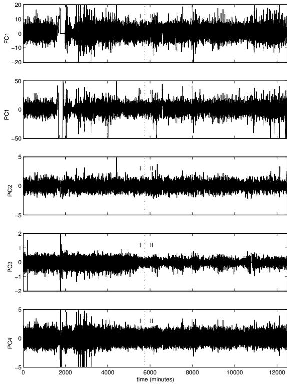
Fig. 2. Time series of setpoint error ( $PV - SP$ ) for five power boiler loops
