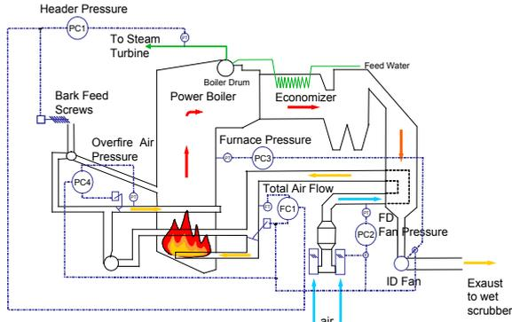
Fig. 1. Power boiler schematic
