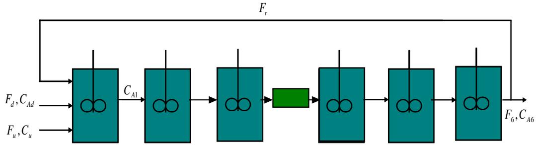
Fig. 1. The schematic for the example of 6 CST mixers in series with a recycle loop
