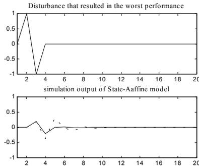
Fig.4. Closed-loop simulations of state-affine model (lower two curves).
