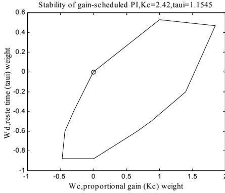
Fig.2. Stability region of gain-scheduled PI controller weights, that is, the area inside the solid box including the solid circle as limit.
