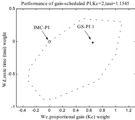
Fig.3. Performance region of gain-scheduled PI controller weights, that is, the area inside the dotted box including the dotted circle as limit.
