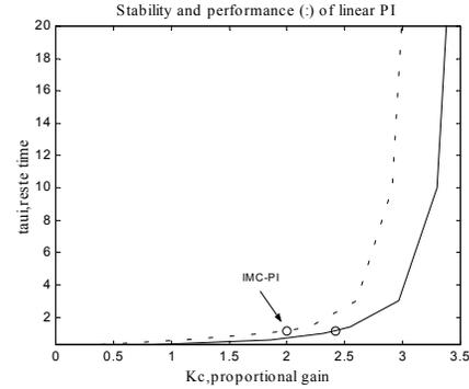
Fig.1. Stability and performance regions of linear PI controller parameters. Stability region is the area above the solid line including the solid line as limit. Performance region for a  $\gamma=1$  is the area above the dotted line including the dotted line as limit.
