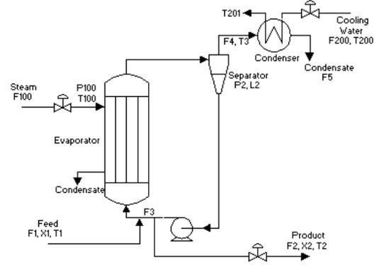
Fig. 1. Evaporator System
