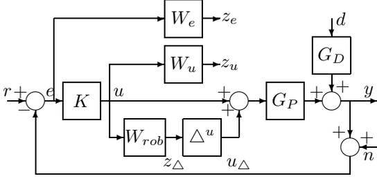
Fig. 2. Block Diagram Describing Weighted System with Multiplicative Uncertainty
