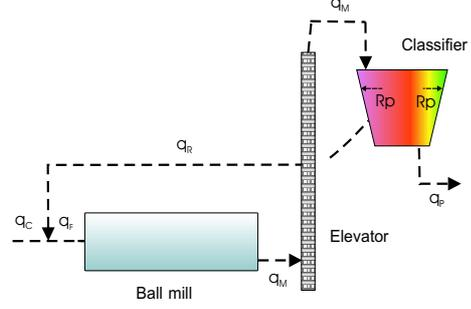
Fig. 1. Closed-loop grinding circuit
