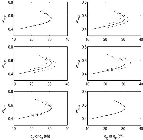
Fig. 6. Parameter sensitivity analysis :  $\alpha_1$  and  $\alpha_2$  (top figures),  $k$  and  $\beta$  (intermediate figures),  $u$  and  $D$  (bottom figures); (dashed)  $-10\%$ , (dash-dotted)  $+10\%$  on the parameter estimate, respectively
