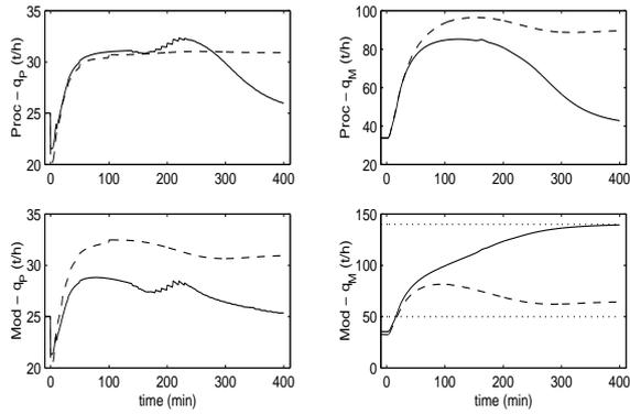
Fig. 8. DMC-like compensation results; (solid):  $C = 0.9$ , (dashed):  $C = 1.1$
