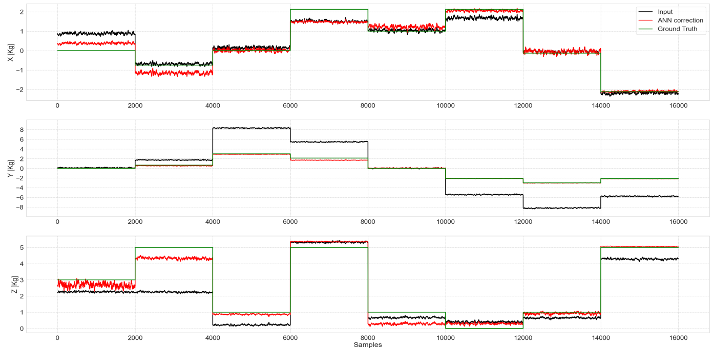
Fig. 6. ANN correction of the artificial signal
