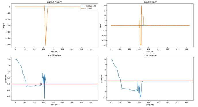
Fig. 1. CE MPC with zero-mean Gaussian process noise:  $v \sim N(0, 0.05)$ . The oscillations in input signals result in a spike in the output, but parameter estimations converge close to true values.
