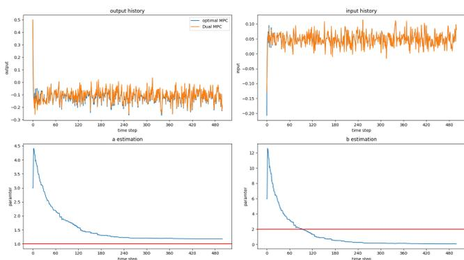
Fig. 4. Dual MPC:  $v \sim \mathcal{N}(-0.1, 0.05)$ . The dual MPC has performance consistent with the optimal MPC.
