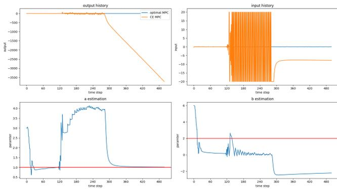
Fig. 3. CE MPC:  $v \sim \mathcal{N}(-0.1, 0.05)$ . The estimation error in  $b$  is present and the CE MPC failed to control the plant to the zero set point.
