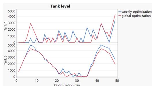
Fig. 8. Tank 1 and 5 level for June 2018 optimization.
