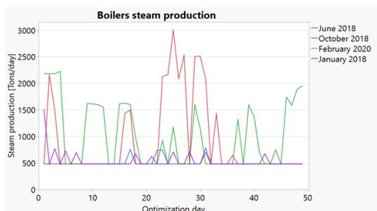
Fig. 7. Steam produced by the boilers in the different periods
