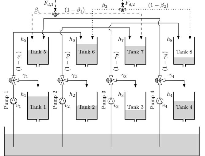
Fig. 1. Schematic diagram of octuple tank system
