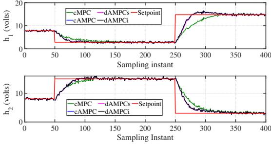
Fig. 2. Comparison of controlled outputs: levels 1 and 2
