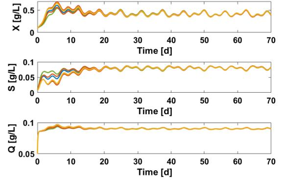
Fig. 7. RLS-ES application: evolutions of the biomass, substrate and internal quota concentrations.
