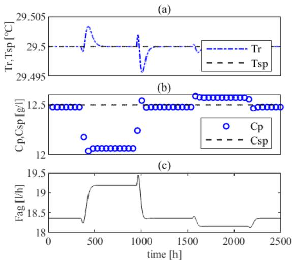
Figure 2. SISO control performances: (a) controlled reactor temperature; (b) ethanol concentration (open loop); (c) manipulated coolant flow rate.
