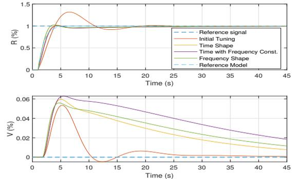
Fig. 4. Reference Step Experiment at Loop 1
