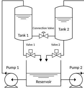
Fig. 6. Coupled Tanks Pilot Plant Schematic
