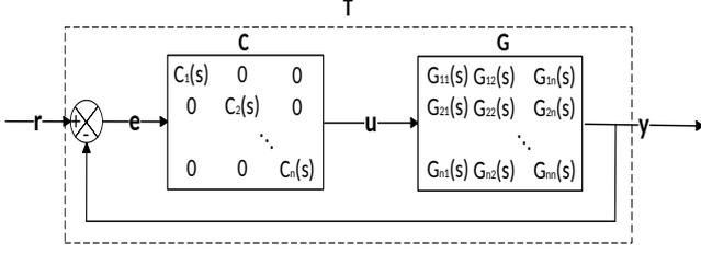
Fig. 1. MIMO Decentralized Closed Loop
