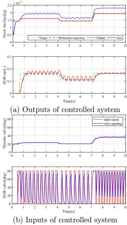
Fig. 3. Simulation results of the method without anti-windup compensation
