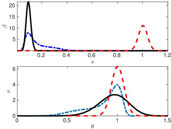
Fig. 4. Stationary marginal substrate PDF  $\bar{\beta}$  (top panel) and stationary control variable PDF  $\nu$  (bottom panel). Initial conditions:  $(m_0, s_0) = (0.9, 0.0901)$ , noise:  $(q_m, q_s) = (0.002, 0.002)$ ,  $q_\theta = 0.004$ ,  $\delta^* = 21.11$ , Set point:  $\bar{s} = 0.0901$ ,  $k = 2$  blue line;  $k = 8$  black line; OL dashed red line.
