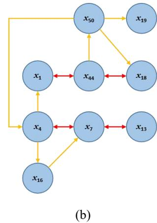
Fig. 6. The causal inference results of the LG method for the TEP example. (a) causality matrix. (b) causality map.
