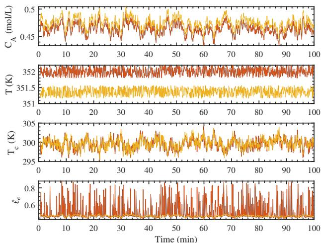
Fig. 4. State, input and economic cost profiles of the CSTR process under tracking MPC (blue), conventional EMPC (red) and our proposed EMPC (yellow)
