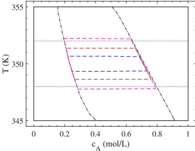
Fig. 1. Effect of risk factor on the economic zone. Hard constraints (black solid), largest robust controlled invariant set (black dash-dot), economic zones (magenta:  $\delta = 50$ , red:  $\delta = 20$ , blue:  $\delta = 10$ ), original zone (black dots)
