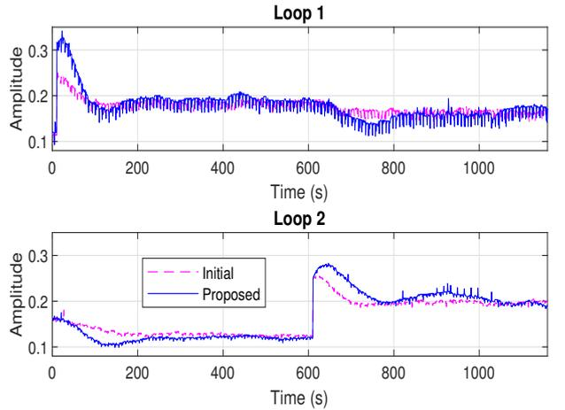
Fig. 9. Initial and proposed control signal - experiment
