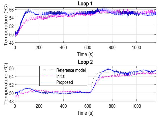
Fig. 8. Closed-loop responses with controllers (40) and (42) - experiment
