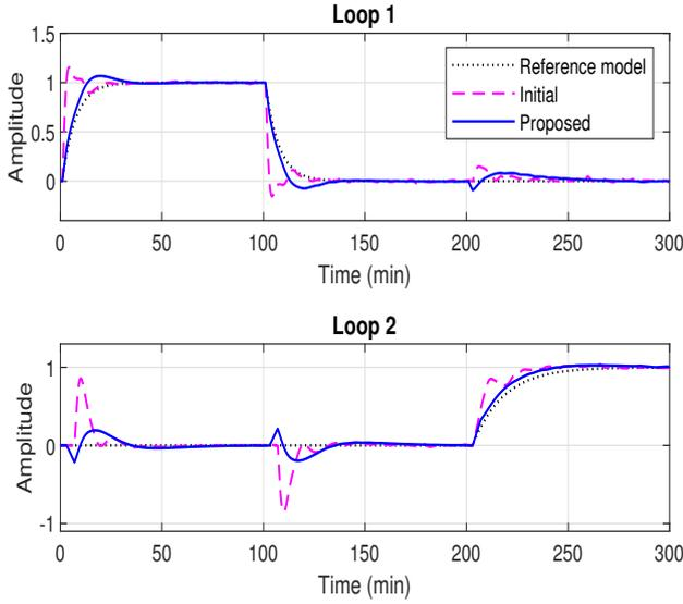
Fig. 3. Closed-loop responses of system (30) with controllers (34) and (35) - initial decentralized controller - example 1
