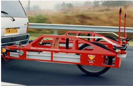
Fig. 4. LCPC experimental vehicle towing the LPA.
