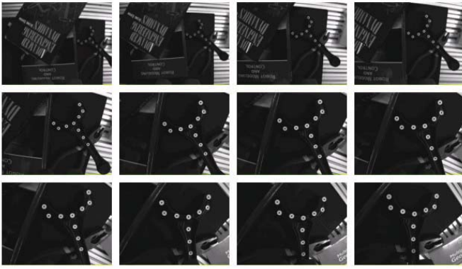
Fig. 12. Sequence of camera motions generated by MPC visual servoing to complete a grasping task. The resulting image feature trajectories satisfy the camera field-of-view constraints.
