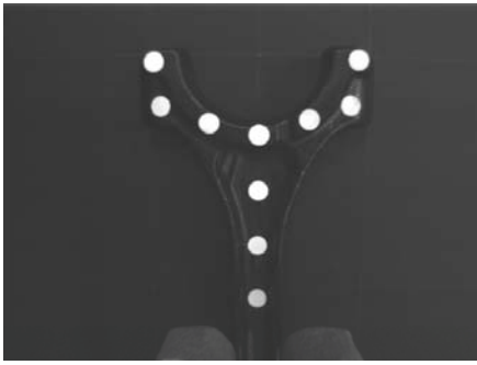
Fig. 2. Reference image describing the desired position of the end-effector with respect to a target object.
