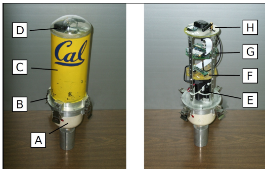
Fig. 1: Overview of the drifter hull. Left: closed. Right: open.
