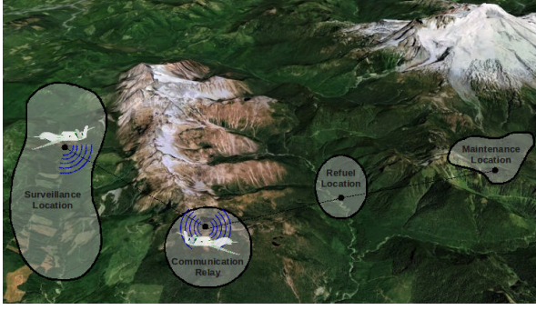
Fig. 1. N agents cooperate to continuously survey a specified region and to track any objects of interest discovered there. This behavior is to be maintained even under sensor and actuator health degradations.
