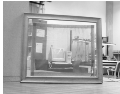
Figure 1: Transparent thin film speaker used in window active noise control system by X. Yu et al.
