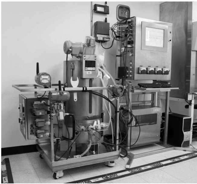
Fig. 14. A single-use-bioreactor (SUB) and bench top reactors with wireless devices and new in-line and at-line analyzers and a lab optimized industrial DCS are being used for control studies in conjunction with a virtual plant.
