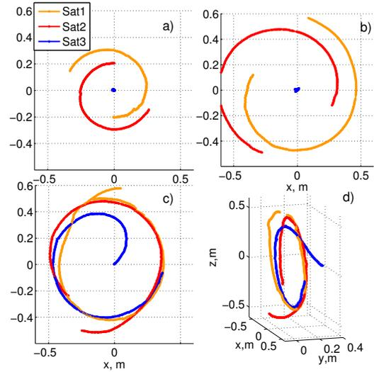
Fig. 4. Experimental results: a) rotation in the  $x$ - $z$  plane; b) convergence to a circle with larger radius; c) the third spacecraft joins the formation; d) 3D plot of third maneuver.
