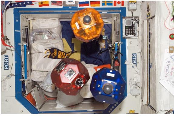
Fig. 2. Picture of the three SPHERES spacecraft performing a test on board the ISS (Fotocredit: NASA-SSL).
