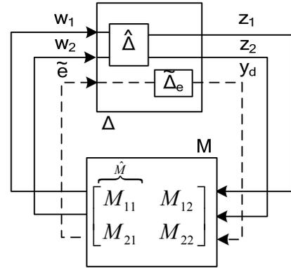
Fig. 3. The  $M$ - $\Delta$  interconnection isolating uncertainty blocks.
