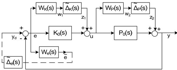
Fig. 2. Expanded control loop with additive uncertainties and a fictitious performance block.
