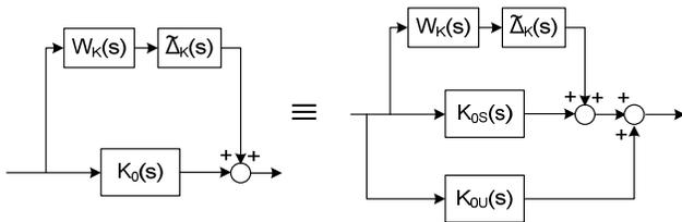
Fig. 4. Separation of stable and unstable controller components
