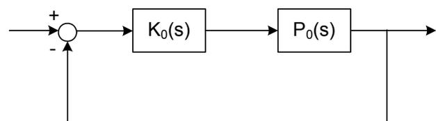
Fig. 1. Typical feedback control system with nominal models for the controller and plant.
