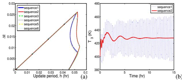
Fig. 3. (a) Dependence of  $\lambda_{\max}$  on the sensor transmission interval  $\Delta t_1$  and the update period for different sensor transmission sequences with a fixed model uncertainty, and (b) Closed-loop temperature profiles for CSTR 3 under the model-based quasi-decentralized control strategy using two different sensor transmission schedules with the same update period.
