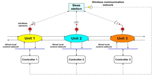
Fig. 1. Quasi-decentralized control structure with cross communication over a plant-wide wireless sensor network.
