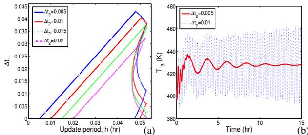
Fig. 4. (a) Dependence of  $\lambda_{\max}$  on  $\Delta t_1$  and  $h$  for different values of  $\Delta t_2$  under sensor transmission schedule 1 with a fixed model uncertainty, and (b) Closed-loop temperature profiles for CSTR 3 when  $\Delta t_1 = 0.01$  hr and  $h = 0.05$  hr for two different values of  $\Delta t_2$ .
