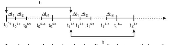
Fig. 2. A schematic showing the time-line for the transmission of each sensor suite in an  $h$ -periodic schedule.
