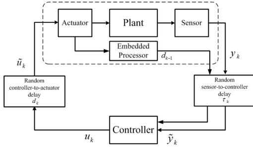
Fig. 1. Diagram of a networked control system.
