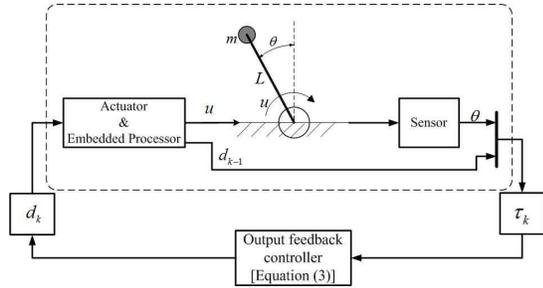
Fig. 2. An inverted pendulum system.
