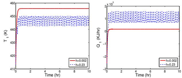
Fig. 2. Closed-loop state and manipulated input profiles for CSTR 1 under the model-based nonlinear quasi-decentralized control strategy with model uncertainty of  $\delta_1 = 0.01$  and different update periods.
