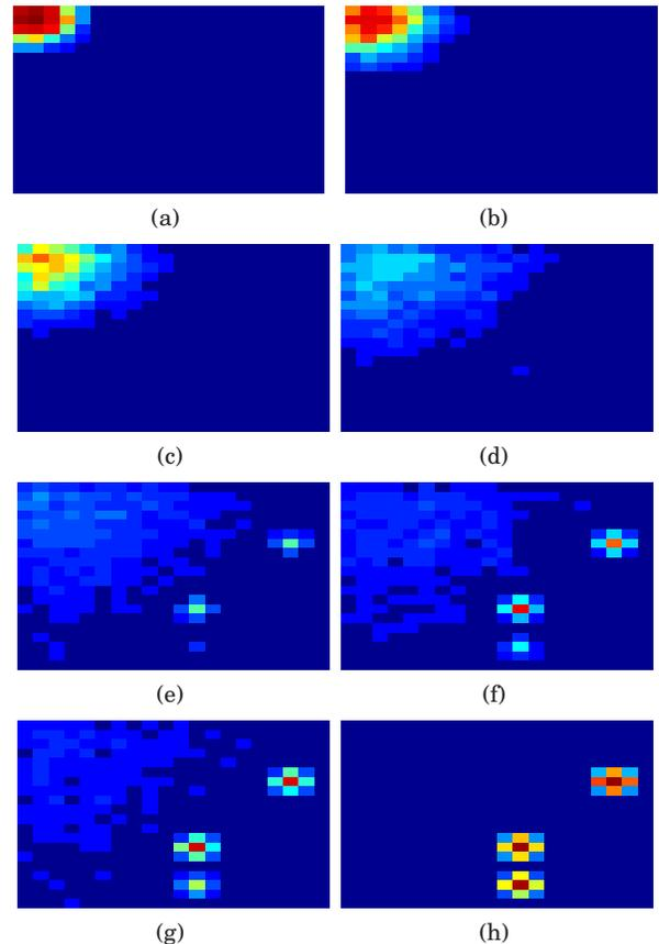
Fig. 4. Self-organization of the Sensor Field subsequent to Control Broadcast. The initial field is concentrated at the top-right corner as seen in (a) which subsequently organizes to peak at the activity hotspots. The spatial convergence is illustrated by the plates (b)-(h). A similar simulation result for a smaller problem can be viewed in the movie form by running the "swarm.avi" supplied as an attachment
