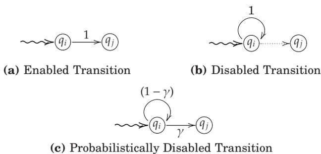
Fig. 1. Probabilistic Disabling of Finite-State Markov Chains
