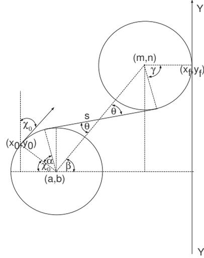
Fig. 2. Dubins' RSL path for initial orientation  $(\chi_0) < \pi/2$  and final orientation  $(\chi_f) = 0$ .
