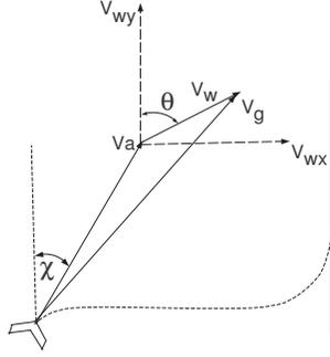
Fig. 8. Representation of airspeed ( $v_a$ ), ground speed ( $v_g$ ) and wind speed ( $v_w$ ).
