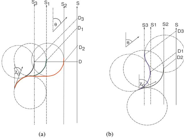
Fig. 9. (a) First quadrant: Wind case for RSL and  $RL^1$  path (b) First quadrant: Wind case for  $RL^1$ , L and  $LR^1$
