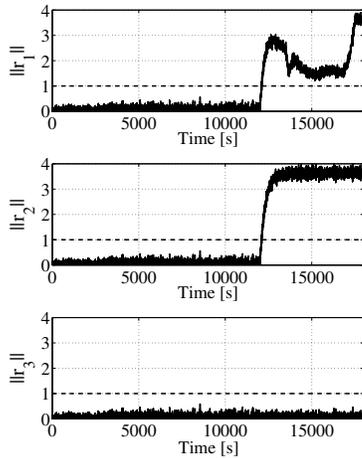
Fig. 3. Sensor  $T_{j,2}$  and cooling system faults: isolation residuals for the actuator fault.
