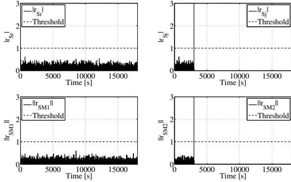
Fig. 1. Sensor  $T_{j,2}$  and cooling system faults: detection and isolation residuals for the sensor fault.
