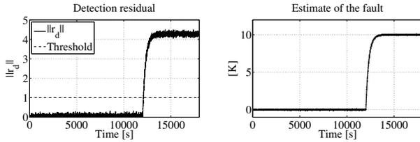
Fig. 2. Sensor  $T_{j,2}$  and cooling system faults: detection residual and estimate of the actuator fault.
