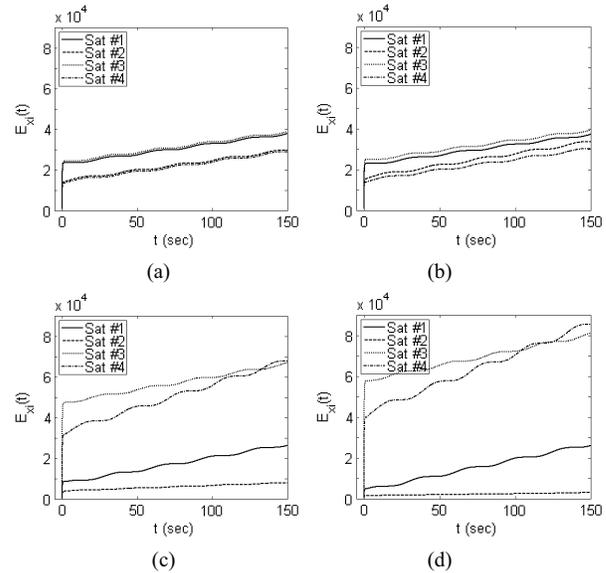
Fig. 2. The x-axis cumulative input effort for (a) the case of all satellites fault free, (b) faulty satellite #2 with LLFR:  $\alpha_2 = 1$ , (c) faulty satellite #2 with HLFR:  $\alpha_2 = 6$ , and (d) faulty satellite #2 with HLFR:  $\alpha_2 = 10$ .
