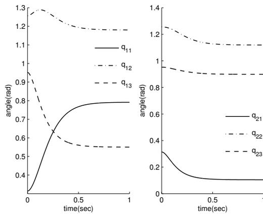
Fig. 5. Transient responses for the angles of the fingers 1 and 2
