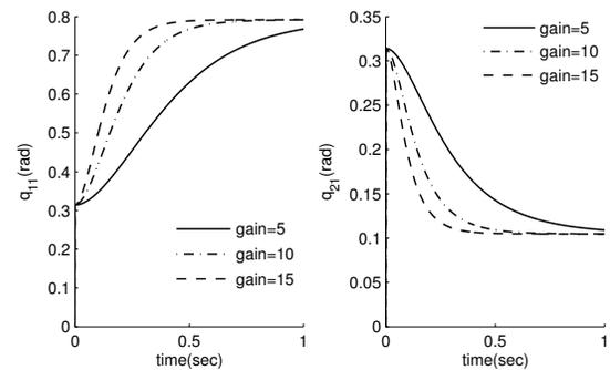
Fig. 8. Transient responses for the first angle of the fingers 1 and 2
