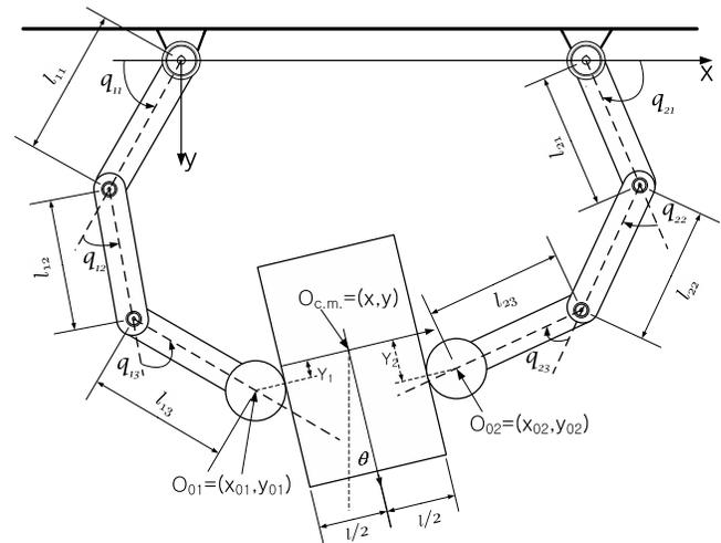
Fig. 1. 3-joint dual finger robot system
