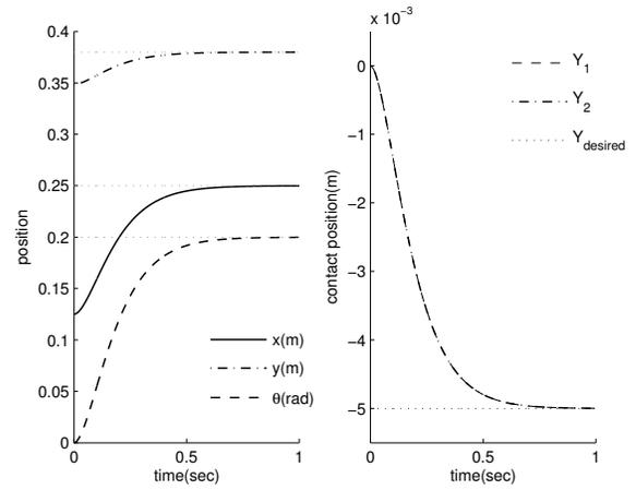
Fig. 6. Transient responses for the center of mass and rolling contact position
