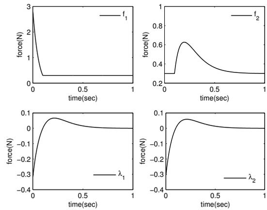
Fig. 7. Normal and tangential contact forces by fingertips
