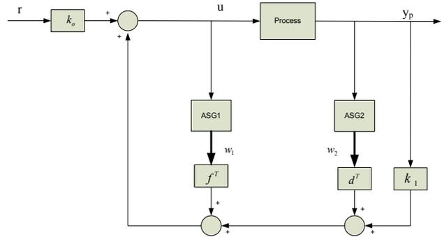
Fig. 2 Primary controller structure of augmented error method
