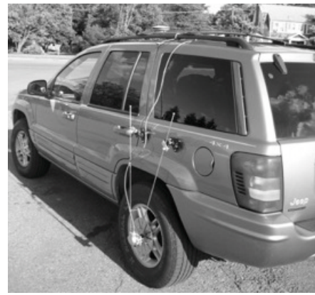
Fig. 2. Side view of the test vehicle shown with the wheel odometry and GPS antenna.
