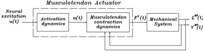
Fig. 1. Block diagram that shows the interaction of tendon and muscle with a mechanical system.
