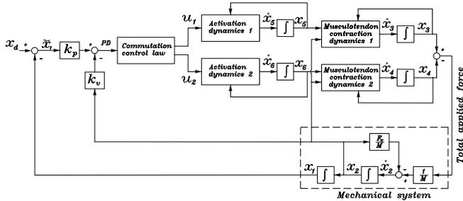
Fig. 3. Block diagram that represents the feedback control system (18).
