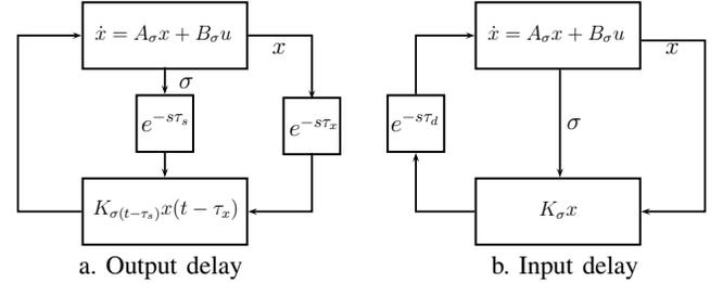
Fig. 1. Feedback switched systems with delays
