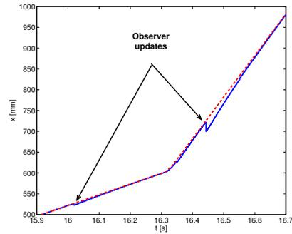
Fig. 8. Experimental results of the ARTC algorithm performing closed loop sheet control in the printing system on-ramps. Figure shows the sheet lead edge desired reference trajectory (dashed) and estimated position (solid). Notice how the estimated position is controlled to track the desired whenever a sheet sensor updates the estimated sheet position.
