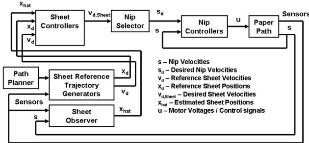
Fig. 3. Overview of the ARTC control architecture.
