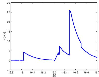
Fig. 9. Experimental results showing the tracking errors from the previous figure, i.e. the difference between the desired sheet LE position ( $x_d$ ) and the estimated position ( $\hat{x}$ ) for the on-ramp ARTC controls. All tracking errors are continuously being removed by the ARTC algorithm.
