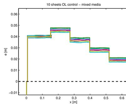
Fig. 12. Sheet tracking errors for Job 2: Mixed media, utilizing open loop control. No removal of errors, range of tracking errors increases from 2.0 to 4.0 mm after 1st bend, at  $x = 0.151$  m, this range is not decreased along the media path.
