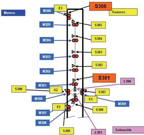
Fig. 10. Output Module used for ARTC performance characterization. Sheets entered output module at entry E1 (upper left) and exited at exit X1 (lower right).
