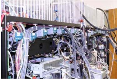
Fig. 6. Close-up of nip motors driving the upper highway nips.
