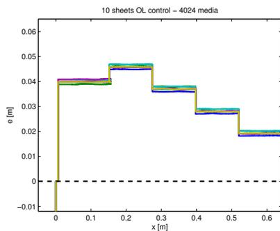
Fig. 11. Sheet tracking errors for Job 1: 4024 - 75 gsm media, utilizing open loop control. No removal of errors, range of tracking errors remains the same along media path.
