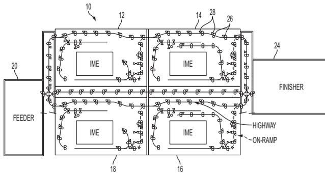
Fig. 1. Overview of a parallel printer architecture. Multiple print engines printing concurrently offer print speed scalability and redundancy. The required large and complex media path presents novel controls challenges.
