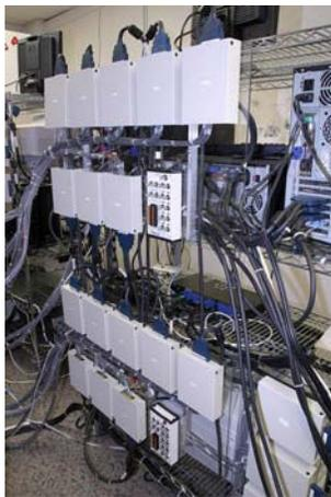
Fig. 7. Hardware implementation of ARTC media path controls utilizing 8 xPC Targets and associated harnessing.
