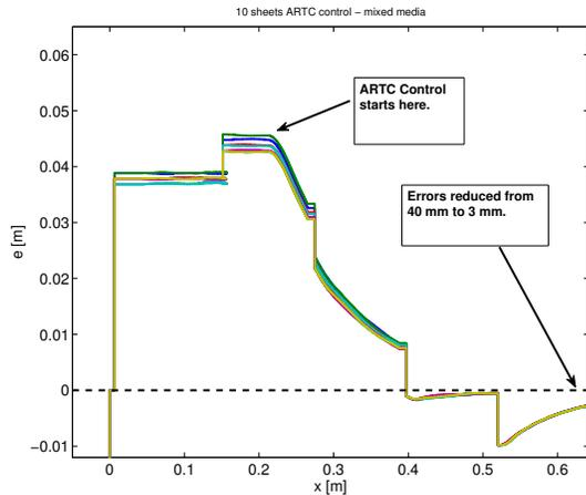
Fig. 13. Sheet tracking errors for Job 3: *Mixed media*, utilizing ARTC control. Both the mean as well as the range of the tracking errors are actively decreased throughout media path by the ARTC algorithm. Compare with figure 13 that utilizes open loop sheet control. On average, incoming errors were reduced from 40 mm to 3 mm and their range was reduced from 4 to 1 mm.
