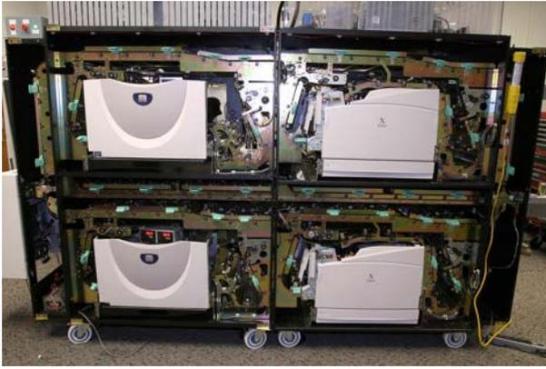
Fig. 5. Four print-engine parallel printing system at the Xerox Research Center, Webster, NY, U.S.A.
