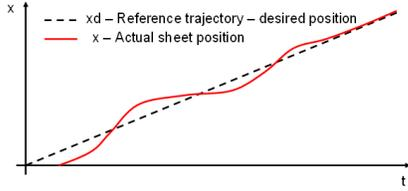
Fig. 2. ARTC — each sheet controlled to track its reference trajectory.
