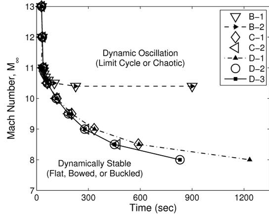
(a) Comparison of flutter boundaries for the aerothermoelastic modeling cases.
