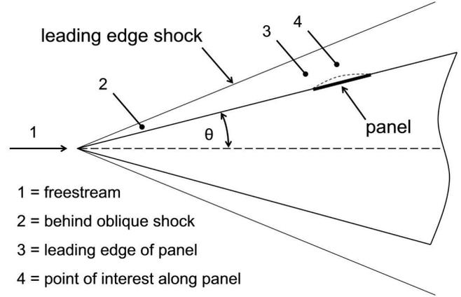
Fig. 3. Panel located on an inclined surface of a wedge-shaped body.
