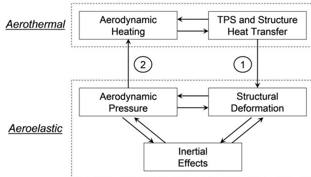
Fig. 2. Fully-coupled modeling approach for aerothermoelastic systems.
