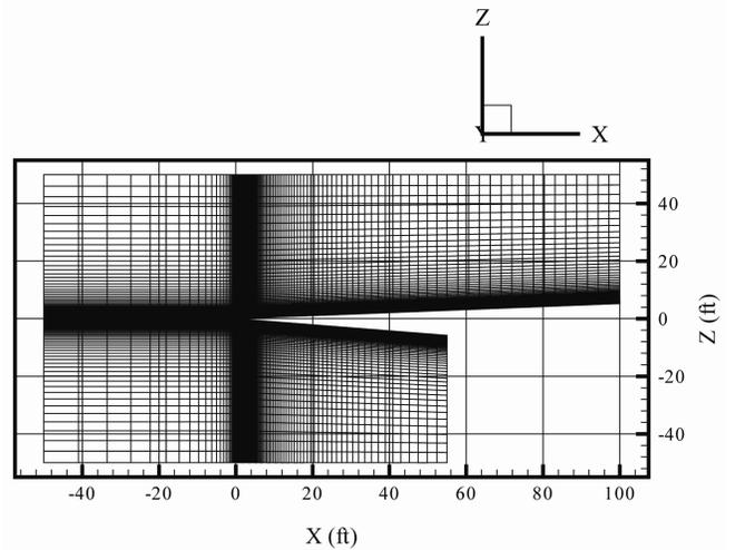
Fig. 5. Computational grid for the forebody of an air-breathing hypersonic vehicle geometry.
