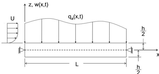
Fig. 4. Simply supported plate structure.
