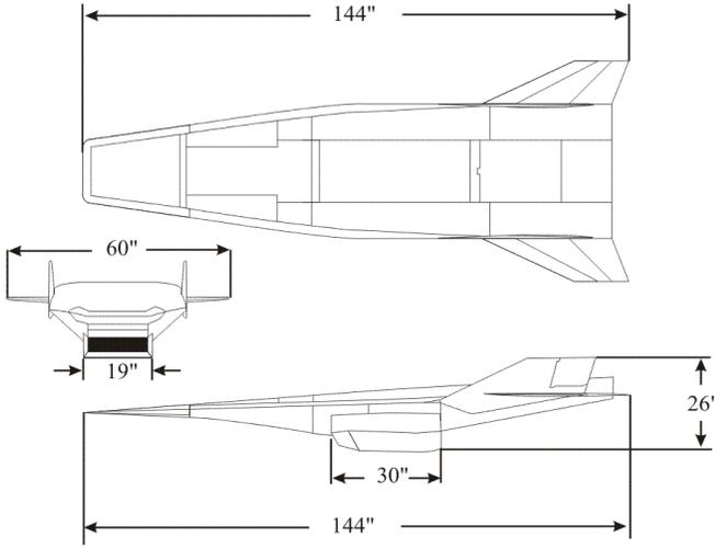
Fig. 1. Schematic of the NASA X-43 Experimental Aircraft.
