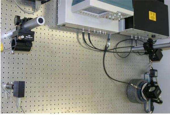
Fig. 1. UCLA laser beam steering experiment. Upper left: laser source. Upper right: FSM 1, disturbance actuator. Lower right: FSM 2, control actuator, mounted on shaker. Lower left: optical position sensor.
