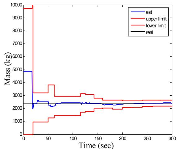
**Figure 6: Mass Estimation Results, Chrysler Proving Grounds**
