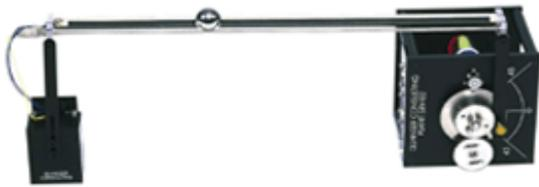
Fig. 2. Ball and Beam Apparatus from Quanser, Inc.
