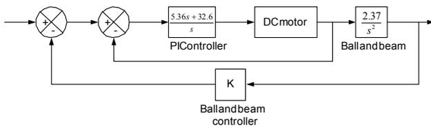
Fig. 3. Closed-loop Ball and Beam System
