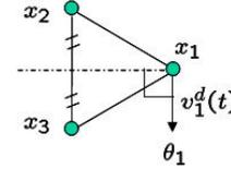
Fig. 4. The desired formation of three agents: The desired relative distances for every two agents are 1.  $z_{32}$  is always aligned with the direction of  $v_1^d(t)$ .
