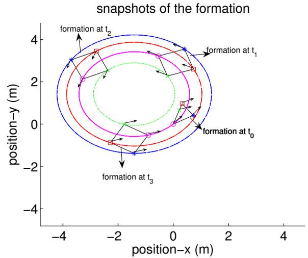
Fig. 7. The desired formation is achieved: The arrow denotes the heading of each agent and initially the headings of all the agents are different. Magenta  $\circ$ , green  $\times$ , red  $\square$  and blue  $*$  represent  $x_1$ ,  $x_2$ ,  $x_3$  and  $x_4$ , respectively.
