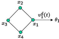
Fig. 6. The desired formation of four agents is a square with side length 1, where  $z_{13}$  is always aligned with the leader's heading  $\theta_1$ .
