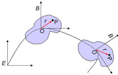
Fig. 1. Rigid body moving along a curve in the 2D space
