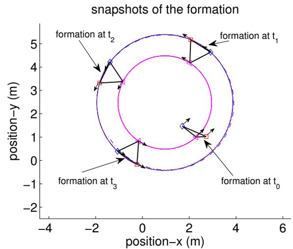
Fig. 5. The desired formation in Figure 4 is achieved: The arrow denotes the heading of each agent and initially the headings of all the agents are aligned. Magenta  $\Delta$ , blue  $\diamond$  and red  $\square$  represent  $x_1$ ,  $x_2$  and  $x_3$ , respectively.
