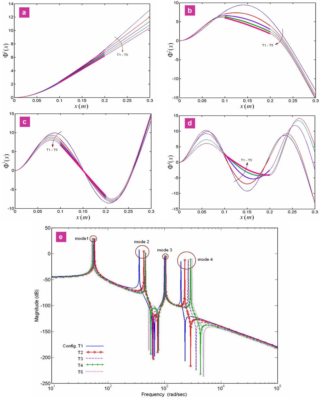
Figure 3. (a) First, (b) second, (c) third, and (d) fourth mode shapes of beams with five different middle section thicknesses, and (e) frequency response plot of beams' tip displacements.
