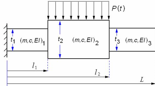
Figure 2. EB beam with two stepped discontinuities in cross section under distributed dynamic load.
