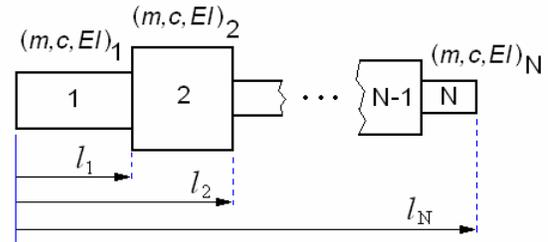
Figure 1. EB beam configuration with  $N$  jumped discontinuities.
